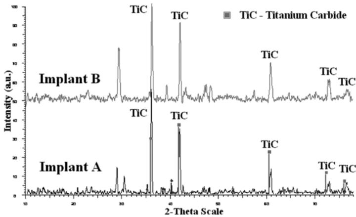
Figure 3. XRD pattern of titanium alloy sintered implants.
