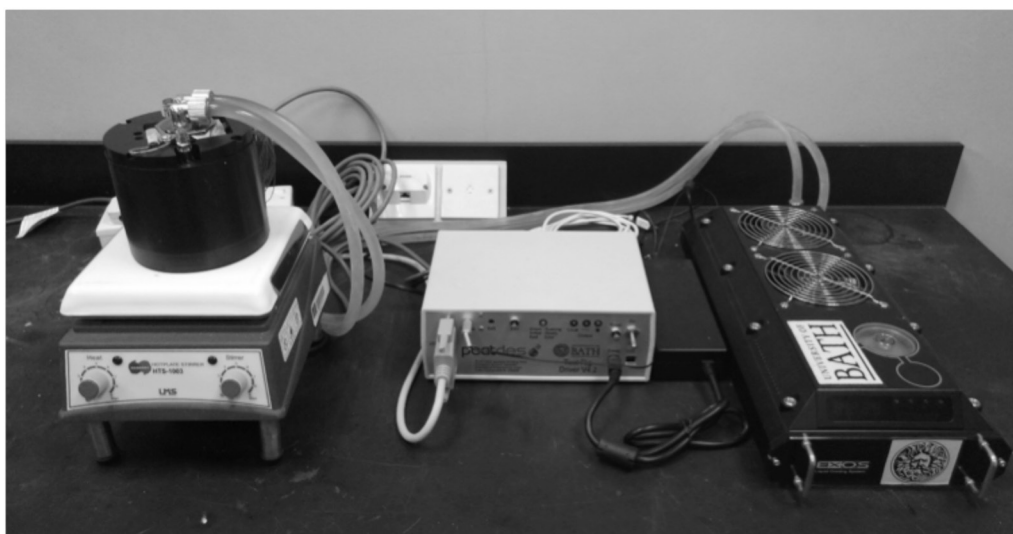
Figure 1. Experimental set-up of the photocatalytic degradation of trans-Cinnamic acid using standard reactor
